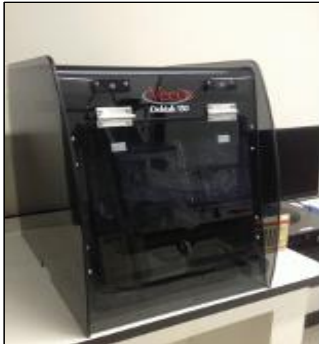
Figure 16 – Contact profilometer from Lamult laboratory – UNICAMP.
