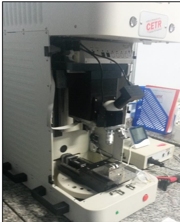
Figure 17 – Tribometer UMT from IP&D - UNIVAP.
