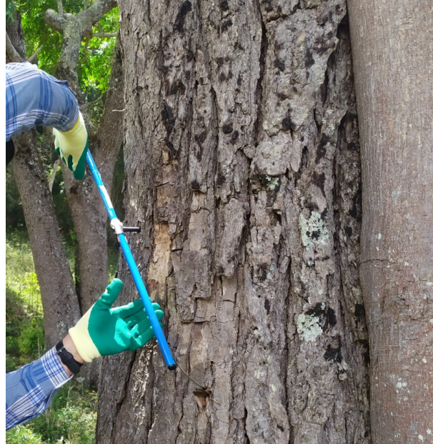
Figure 21: Sample extraction using a Pressler Probe.
