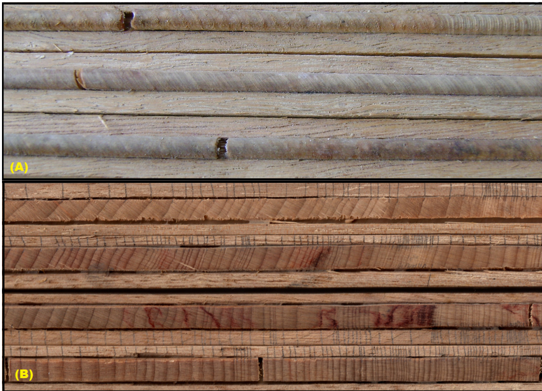
Figure 22: (A) Samples before being polished and (B) sanded, polished and marked samples.
