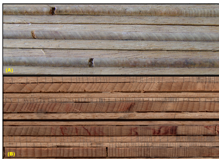
Figure 5. Panel (A) demonstrates the initial state of the cores. The cores extracted by the increment borer are cylindrical in shape, preserving the cross-sectional structure of the tree rings, which allows for accurate dendrochronological analysis after proper preparation and mounting. Panel (B) shows the properly sanded and mounted samples, highlighting the tree-ring boundaries. Source: Natural Records Laboratory (LRN).
