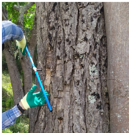
Figure 4. Sample extraction using a Pressler Probe. Source: Natural Records Laboratory (LRN).
