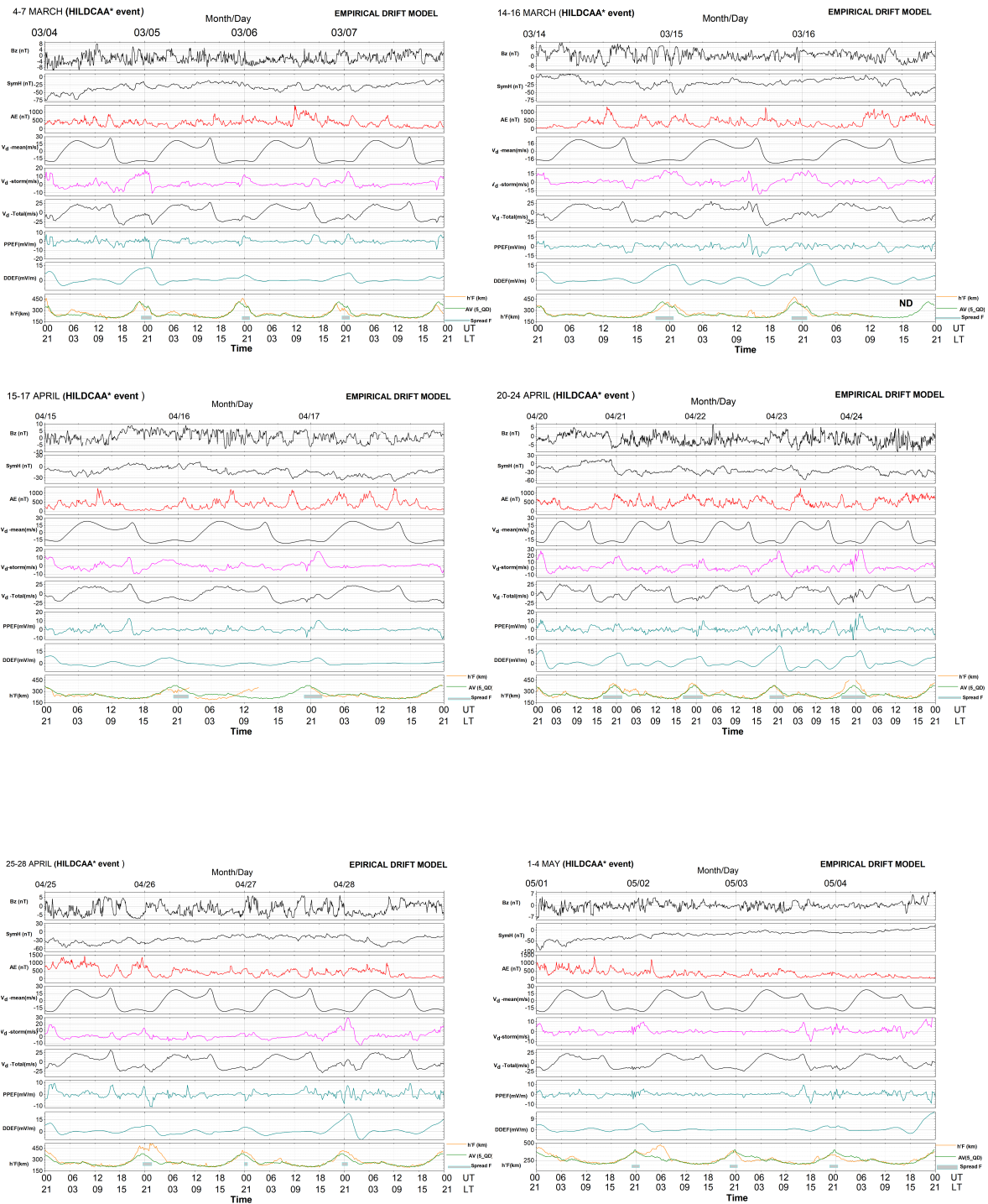
Figure A.30 – Variations of interplanetary magnetic field ( B_z ) in (nT), symmetric disturbance index (Sym-H) in (nT), auroral electrojet index (AE), empirical calculation of V_d -mean, V_d -storm, V_d -total, Prompt penetration (PPEF) and Disturbance dynamo drifts (DDEF) drifts components derived from our high time resolution model and ionospheric parameters, h'F (F layer virtual height) including the five quiet days average during the HILDCAA events on 04-07 March, 14-16 March, 15-17 April, 20-24 April, 25-28 April and 1-4 May in 2003
