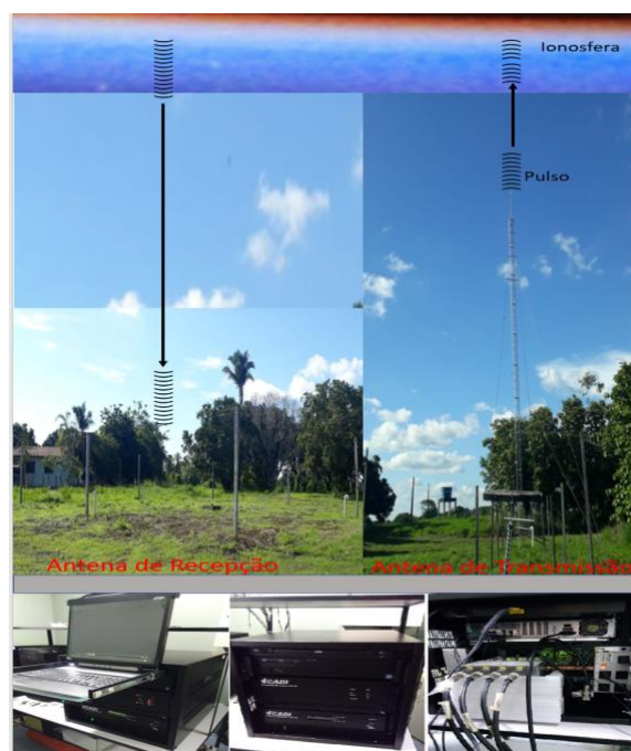
Figure 13 - Transmit antenna system (right side) and reception (left side) of the ionosonde installed in Araguatins with the transmission and reception system (below), respectively.
