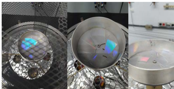
Figure 16 – Three different angular pictures of PC substrate from DVD-R before the sputtering deposition.
