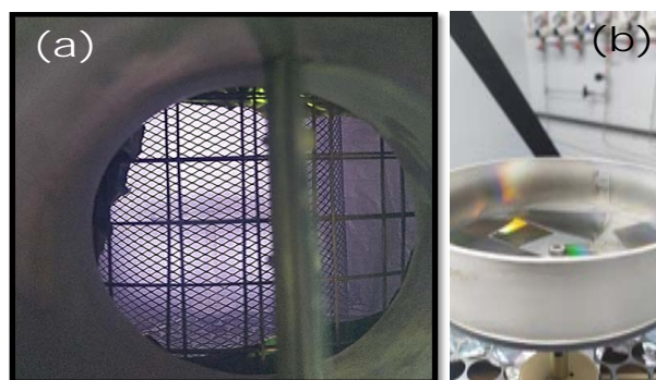
Figure 17 – (a) The argon gas plasma during the deposition process and (b) PC substrate from DVD-R after the sputtering deposition.
