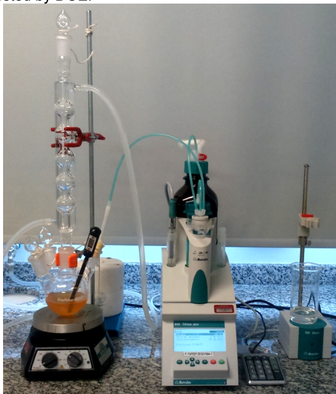
Figure 1.13 – Experimental set-up for coprecipitation of iron oxide nanoparticles, based on the runs suggested by DOE.
