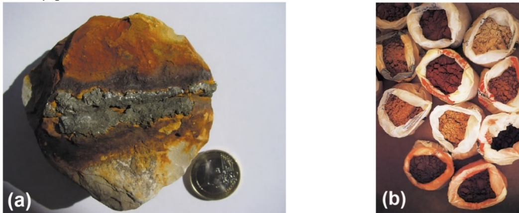
Figure 1.1 – Representation of iron oxides: (a) formation on limestone and (b) iron oxides natural pigments.
