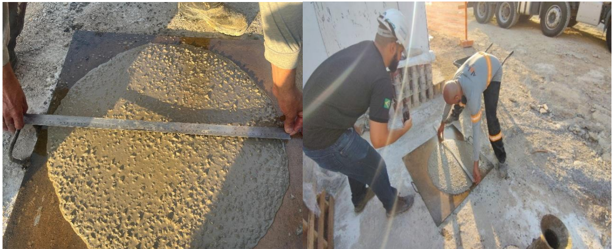
Figura 14 – Slump flow concreto
